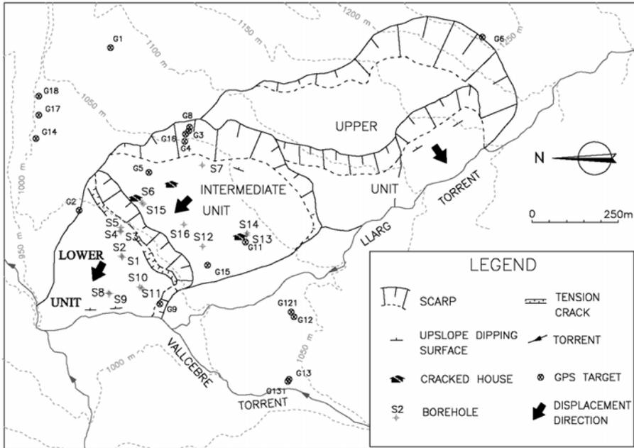
Figure 12. Geomorphological sketch of the Vallcebre landslide. The location of the boreholes and targets of GPS surveying is shown as well (Corominas et al. 1999).
