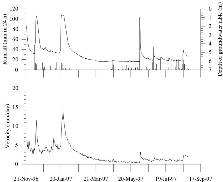
Figure 14. Above: rainfall (bars) and groundwater table changes at borehole S2. Below: rate of landslide displacement from wire extensometer readings at the same borehole (Corominas et al. 1999).
