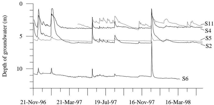
Figure 15. Piezometric records at the Vallcebre landslide.
