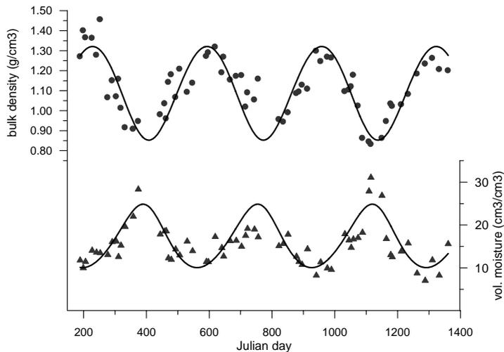
Figure 5: Regolith bulk density and moisture temporal evolution, symbols are measured values from samples and continuous lines represent modelled values (Regüés, 1995)
