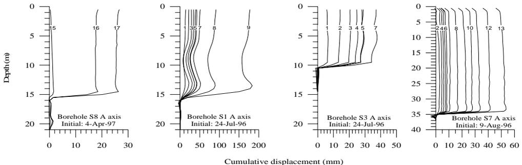
Figure 13. Inclinometric profiles. Numbers in profiles indicate campaign (i.e. number 7 was in 29-Oct-96) (Corominas et al. 1999b).
